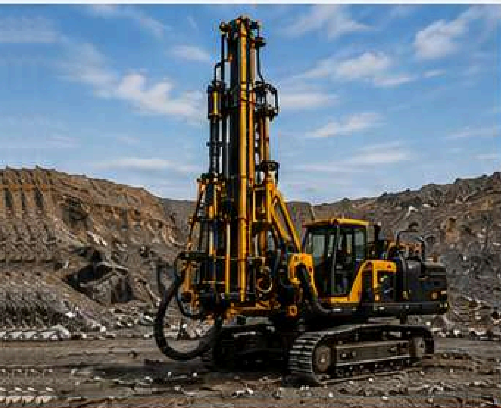
SURFACE DRILLING RIG
