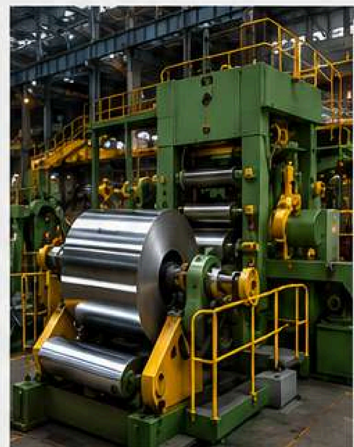
COLD ROLLING MILL
