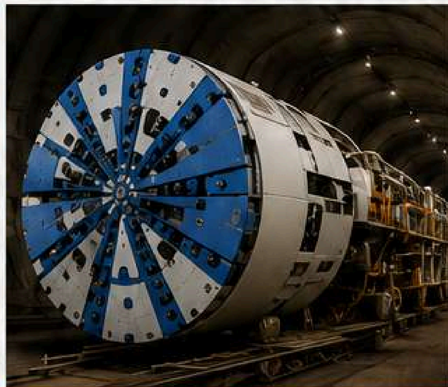
TUNNEL BORING MACHINE
